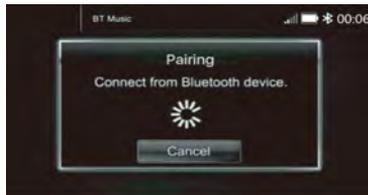
Turn on the Bluetooth of the Mobile phone/ Bluetooth device; you can see the **"SOUNDSTREAM HD"**. Select the **"SOUNDSTREAM HD"** for pairing and connection.
