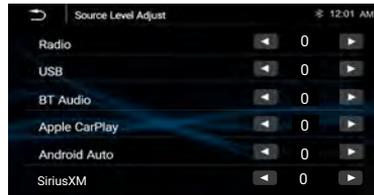
User can adjust the source mode (Radio, USB, BT Audio, Apple CarPlay, Android Auto, SiriusXM) gain value. The gain can be adjusted from -10~0 seperately.
