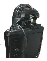
5. Thread the speaker wire thru a hole in the back of the speaker pod removed in step #3. Leave about 3" of speaker wire inside the speaker pod, and 3" between speaker pod and the lower fairing.
