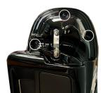
4. Thread the speaker wire included with this kit thru a hole in the sidewall of the lower fairing, located near the crash bar channel. Insert the speaker wire terminals first, pulling about 6" of speaker wire into the fairing. Insert one side of the rubber grommet thru the hole into the fairing.
