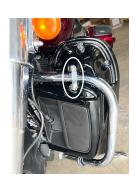
10. Align the screw hole of the lower crash bar clamp to the hole in the bottom of the lower fiaring. Push a lower crash bar clamp hex bolt with washer included in the kit thru the hole in the lower portion of the fairing and thru the holes of the lower crash bar clamp installed in step 8.
