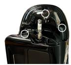
7. Using a ratchet with a 10mm socket on an extension, remove two nuts from the upper crash bar clamp. Set the complete fairing assembly & upper crash bar clamps aside.
