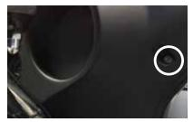
4. Reinstall the windshield & outer fairing to the inner fairing with the three screws removed previously using a T27 Torx screw driver.
