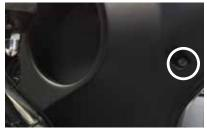
3. While straddling the front wheel fender, grasp the outer fairing. Remove the center windshield screw. Gently pull the fairing apart from the bike. With the fairing slightly pulled away from the bike, disconnect wire harness for the headlight or any other accessories. Lay the fairing on a protected flat surface to prevent damage.
