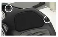
3. Reattach each turn signal / indicator light by installing the two previously removed bolts, located between the fairing and forks using a 1/2" wrench.
