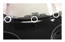
2. Remove four fairing screws holding the outer fairing to the inner fairing using a T27 Torx screw driver. Two screws are located under the fairing adjacent to the forks, two others are adjacent to each speaker. Set screws aside for installation later.
