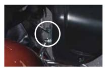
2. Remove six fairing screws holding the outer fairing to the inner fairing using a T25 Torx screw driver. Two screws are located below each glove box, two are adjacent & below each speaker, two others are adjacent & above each speaker. Set screws aside for installation later.
