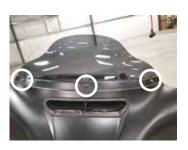
**TIP:** Reinstalling the center screw after removing the windshield will prevent the outer fairing from falling during the next step. A few turns by hand will be sufficient.
