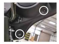
3. Reset the windshield and reinstall the three outer fairing bolts removed previously using a T27 Torx screw driver. The three outer fairing bolts are located below the windshield.
